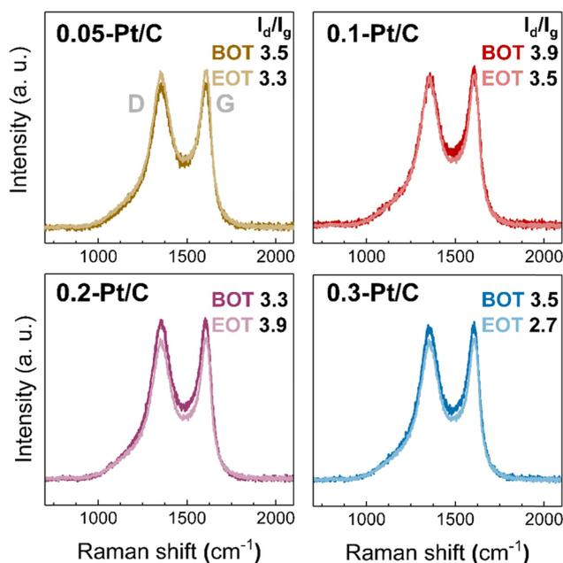
**Fig. 8** Raman spectra for 0.05-Pt/C, 0.1-Pt/C, 0.2-Pt/C and 0.3-Pt/C cathode CLs at beginning of test (BOT) and end of test (EOT) coupled to their respective  $I_{\text{d}}/I_{\text{g}}$  ratio.
