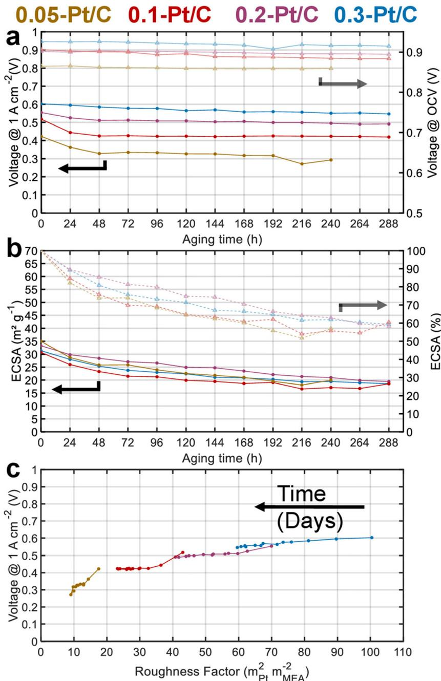
**Fig. 2** (a) Cell voltages measured at 1 A cm<sup>-2</sup> during the daily characterization step and their OCV in the course of the AST; (b) ECSA mapping and its percentage loss; (c) cell voltage at 1 A cm<sup>-2</sup> vs. roughness factor, R.F., both values being measured in real-time along the 288 h of AST for 0.05-Pt/C, 0.1-Pt/C, 0.2-Pt/C and 0.3-Pt/C cathode CLs.
