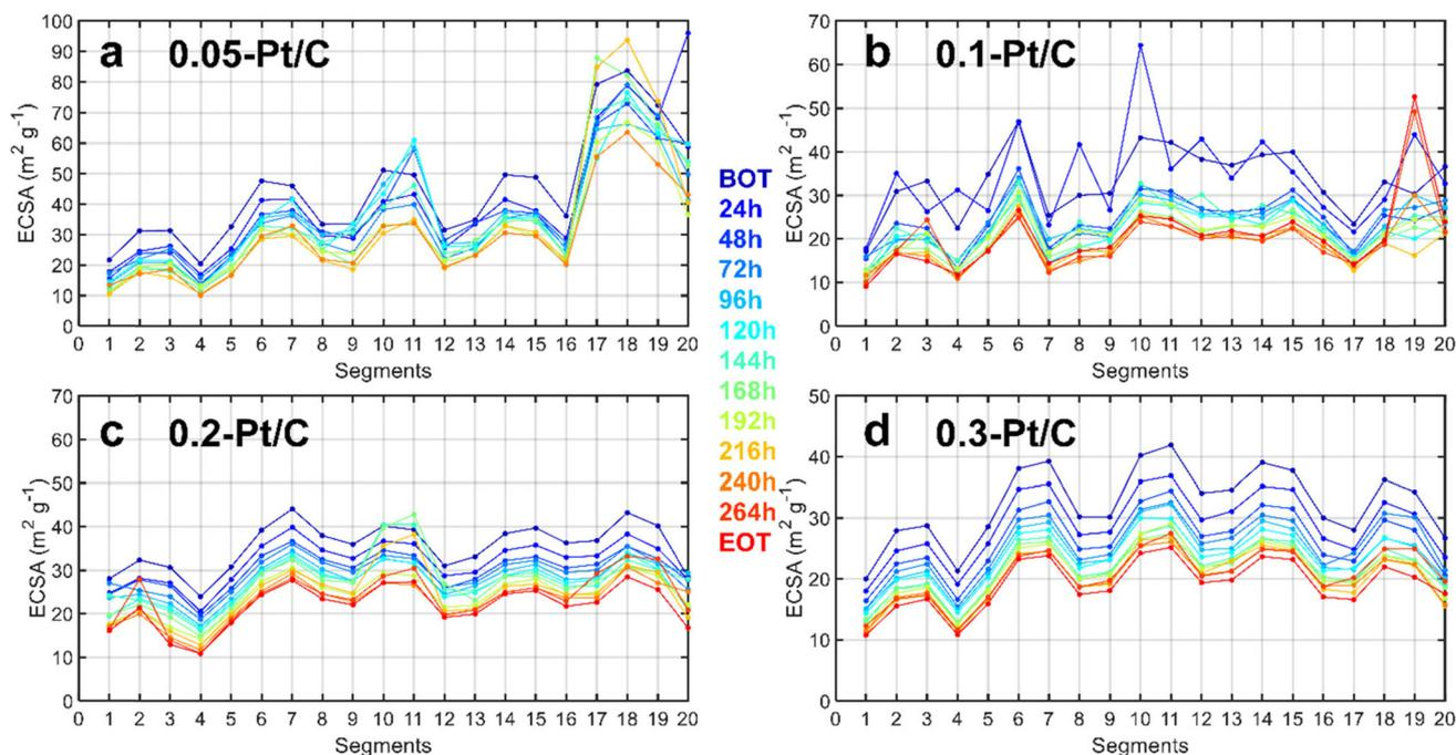
**Fig. 3** Local ECSA along the gas channel measured in a segmented cell for CLs (a) 0.05-Pt/C; (b) 0.1-Pt/C; (c) 0.2-Pt/C and (d) 0.3-Pt/C. Segment #1 corresponds to the air inlet at the cathode and  $\text{H}_2$  outlet at the anode, while segment #20 corresponds to the air outlet at the cathode and  $\text{H}_2$  inlet at the anode.
