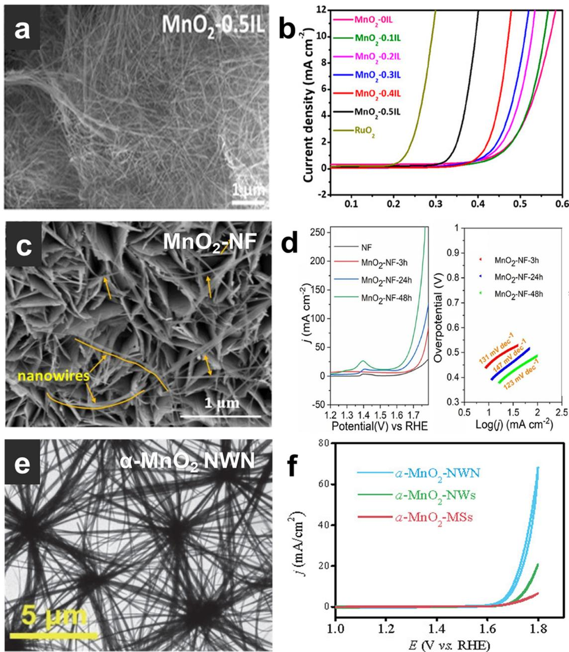
Fig. 5 (a) (c) and (e) TEM images of  $\text{MnO}_2$ -0.5IL,  $\text{MnO}_2$ -NF, and  $\alpha$ - $\text{MnO}_2$  NWN. (b) (d) and (f) Electrocatalytic OER performance of  $\text{MnO}_2$ -0.5IL,  $\text{MnO}_2$ -NF, and  $\alpha$ - $\text{MnO}_2$  NWN. Reprinted with permission from ref. 85. Copyright 2018, ACS Catal. Reprinted with permission from ref. 59. Copyright 2022, *Chem. Eng. J.* Reprinted with permission from ref. 86. Copyright 2021, *Chin. J. Catal.*
