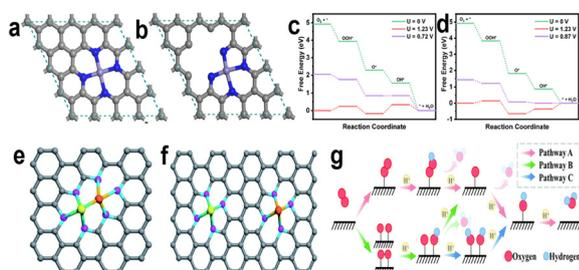
Fig. 2 Model structures used in theoretical studies: (a) center and (b) defective-edge  $\text{FeN}_4$  structures. ORR free-energy diagrams of the (c) center and (d) defective-edge  $\text{FeN}_4$  structures.<sup>18</sup> Model structure of dual-metal catalysts: (e) bonded dual-metal catalysts and (f) non-bonded dual-metal catalysts.<sup>19</sup> (g) Schematic diagram of the reaction pathway of dual-metal catalysts.<sup>20</sup>
