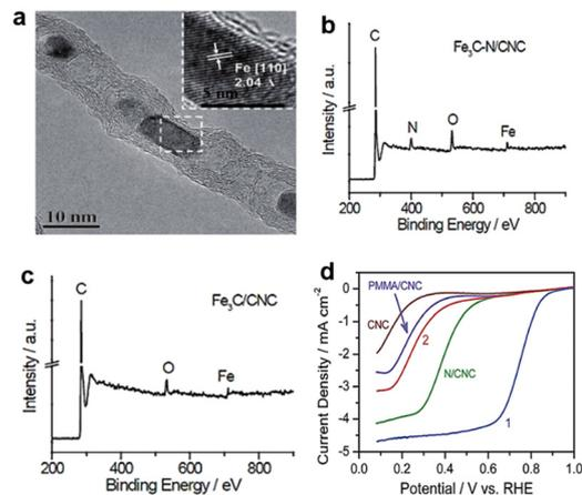
**Fig. 4** (a) High resolution transmission electron microscopy (HRTEM) image of Pod-Fe with the inset showing the [110] crystal plane of Fe.<sup>25</sup> XPS spectra of (b)  $\text{Fe}_3\text{C}-\text{N}/\text{CNC}$  and (c)  $\text{Fe}_3\text{C}/\text{CNC}$ .<sup>29</sup> (d) ORR performance of  $\text{Fe}_3\text{C}-\text{N}/\text{CNC}$  (curve 1) and  $\text{Fe}_3\text{C}/\text{CNC}$  (curve 2).<sup>29</sup>
