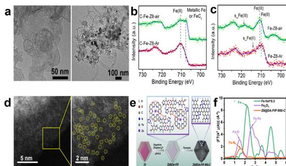
**Fig. 6** (a) TEM images of C-Fe-Z8-Ar (left) and C-Fe-Z8-air (right).<sup>44</sup> (b) High resolution Fe 2p XPS spectra of C-Fe-Z8-Ar and C-Fe-Z8-air.<sup>44</sup> (c) XPS spectra of Fe-Z8-Ar and Fe-Z8-air (without carbonization).<sup>44</sup> (d) AC HAADF-STEM images of Z8@DA-FIP-950-C.<sup>18</sup> (e) Illustration of the synthesis of Z8@DA-FIP-950-C.<sup>18</sup> (f) FT Fe K-edge EXAFS spectra of Z8@DA-FIP-950-C and references.<sup>18</sup>
