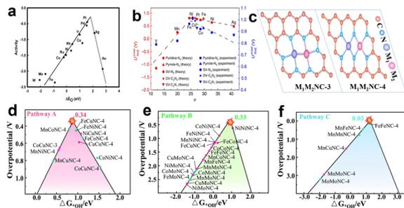
**Fig. 3** Volcanic plot relationship (a) between oxygen reduction activity and oxygen binding energy for various metals<sup>23</sup> and (b) between theoretical and experimental onset potentials ( $U_{\text{onset}}^{\text{RHE}}$ ) versus the descriptor  $\phi$  for single TM atoms supported on graphene.<sup>24</sup> (c) Structural diagrams of  $M_1M_2\text{NC}-3$  and  $M_1M_2\text{NC}-4$ .<sup>20</sup> (d–f) Volcano plots of the three reaction pathways.<sup>20</sup>
