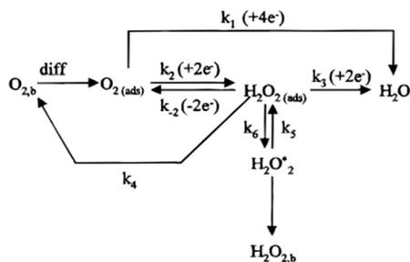
Fig. 1 Schematic diagram of the ORR process under acid conditions.<sup>16</sup>
