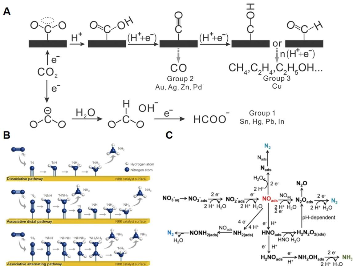
Fig. 2 (A) The possible pathways of multi-step activation and transformation of CO<sub>2</sub> to various value-added products. Reprinted with permission from ref. 15. Copyright 2016, John Wiley & Sons, Inc.; Proposed roadmap of multi-step electroreduction of (B) N<sub>2</sub> and (C) NO<sub>3</sub><sup>-</sup> towards NH<sub>3</sub> synthesis. Reprinted with permission from ref. 22 and 23. Copyright 2019, Elsevier and Copyright 2021, the Royal Society of Chemistry.
