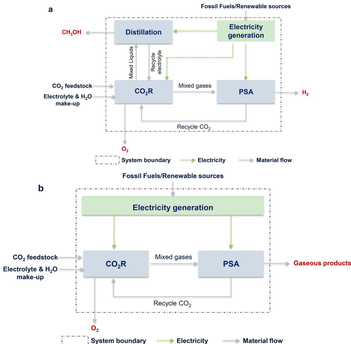
Fig. 7 System boundary for the CO<sub>2</sub>R to CH<sub>3</sub>OH (a) and gaseous products (b).
