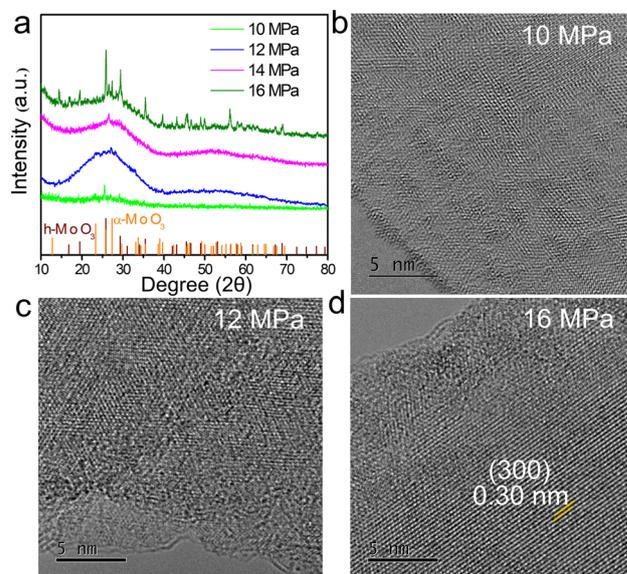
**Fig. 4** (a) XRD patterns comparison of the  $\text{MoO}_{3-x}$  obtained at different pressures, and XRD patterns at the bottom show  $\alpha\text{-MoO}_3$  (JCPDS No. 05-0508) and  $h\text{-MoO}_3$  (JCPDS No. 21-0569); (b–d) HRTEM images of the  $\text{MoO}_{3-x}$  sample obtained at 10 MPa, 12 MPa, 16 MPa.
