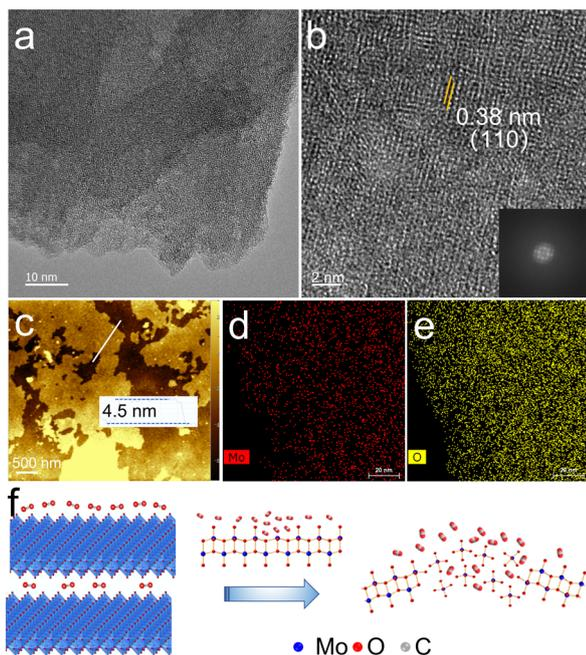
**Fig. 1** (a) TEM image of the  $\text{MoO}_{3-x}$  nanosheets; (b) HRTEM image of the  $\text{MoO}_{3-x}$  nanosheets, inset: the corresponding fast Fourier transform (FFT) pattern; (c) AFM image of the  $\text{MoO}_{3-x}$  nanosheets; (d and e) elemental mapping of the  $\text{MoO}_{3-x}$  nanosheets for Mo and O; (f) schematic side views showing the formation of  $\text{MoO}_{3-x}$  using SC  $\text{CO}_2$ . Mo, O, and C atoms are represented by balls in blue, red, and grey, respectively.
