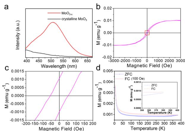
**Fig. 3** (a) PL emission spectra at 300 K of the  $\text{MoO}_{3-x}$  nanosheets and crystalline  $\text{MoO}_3$  excited at 365 nm; (b) magnetization hysteresis loop of the  $\text{MoO}_{3-x}$  nanosheets at 300 K; (c) the magnified curves near  $H = 0$ ; (d)  $M-T$  curves of the  $\text{MoO}_{3-x}$  nanosheets measured under ZFC and FC ( $H = 100$  Oe) modes.
