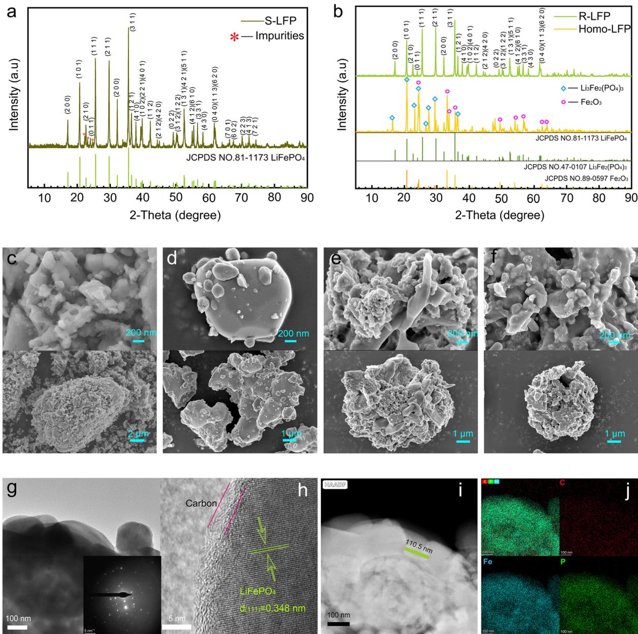
**Fig. 2** Phase analysis and morphological characterization of samples. XRD patterns of (a) S-LFP, (b) Homo-LFP and R-LFP; SEM images of (c) S-LFP, (d) Homo-LFP, (e) spray-dried LFP and (f) R-LFP; (g and h) TEM images of R-LFP; (i and j) HAADF-STEM image and EDS elemental mappings of R-LFP.
