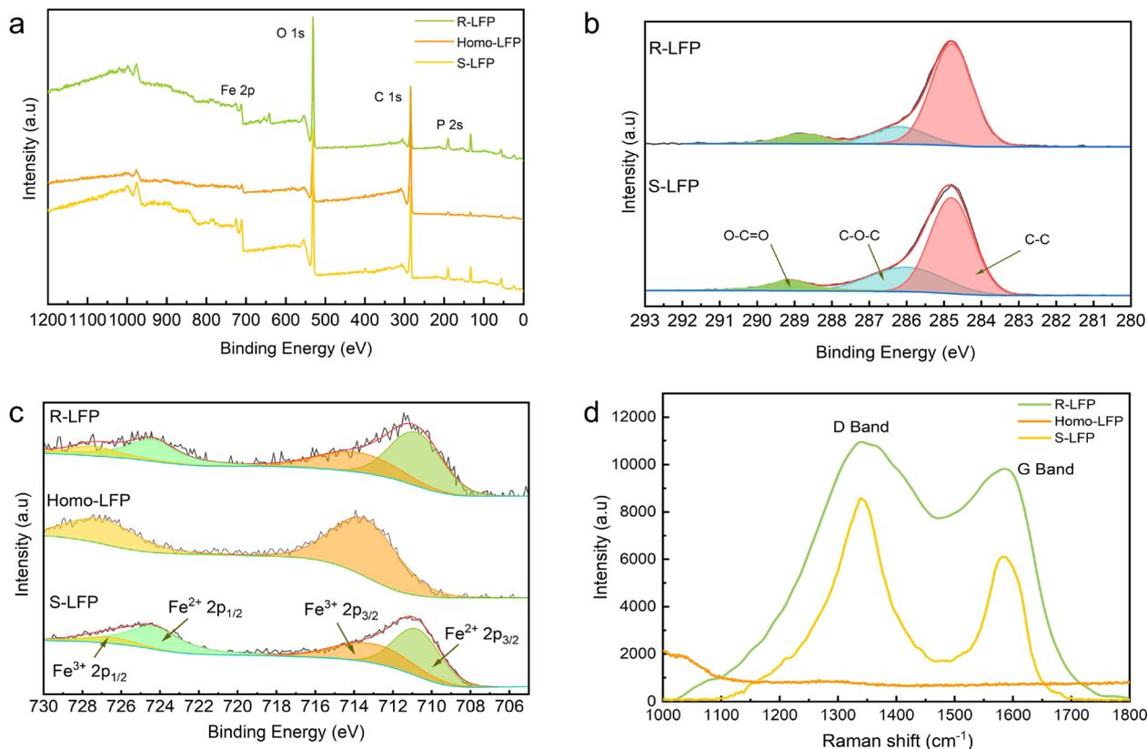
**Fig. 3** XPS and Raman spectra of the samples. (a) XPS survey spectra for the samples; high-resolution spectra of (b) C 1s and (c) Fe 2p; (d) Raman spectra of the samples.
