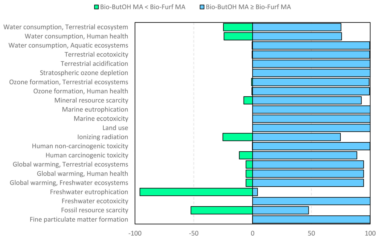
Fig. 9 Uncertainty analysis of bio-based MA routes: the single score impact of each impact category using the ReCiPe 2016 method (v.1.1). Monte Carlo simulation (1000 runs).
