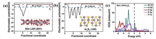
Fig. 22 The electrostatic potentials of (a) Niln-LDH and (b) In<sub>2</sub>S<sub>3</sub>, and (c) the DOS of Niln-LDH/In<sub>2</sub>S<sub>3</sub> (Figures taken with permission from ref. 21 copyright 2023, Elsevier).
