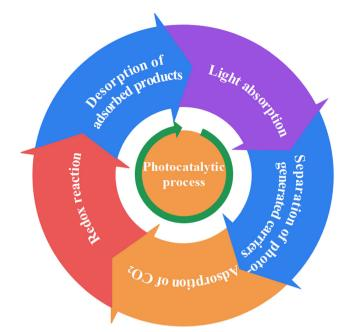
Fig. 2 The photocatalytic process of CO<sub>2</sub> reduction
