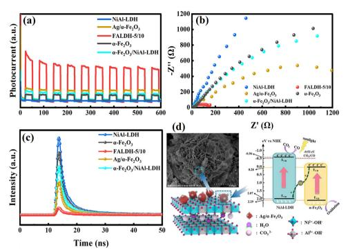
Fig. 19 (a) Photocurrents, (b) EIS spectra, (c) time-resolve fluorescence decay spectra, and (d) the mechanism diagram of FALDH-5/10 (Figures taken with permission from ref. 180 copyright 2023, Elsevier).
