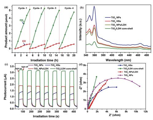
Fig. 18 (a) Recycling tests of CH<sub>4</sub> and CO evolution over the TiO<sub>2</sub>/LDH core-shell hybrid, (b) steady-state PL spectra, (c) photocurrent responses, and (d) EIS profiles of the TiO<sub>2</sub> NPs, TiO<sub>2</sub> HSs, TiO<sub>2</sub> NPs/LDH, and TiO<sub>2</sub>/LDH core-shell hybrid sample (Figures taken with permission from ref. 174 copyright 2023, RSC).
