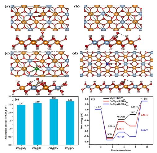
Fig. 14 Optimized structural models of CO<sub>2</sub> adsorption over (a) Mg, (b) Al, (c) Co and (d) Cr sites (Atoms in different colors: yellow-Mg, light blue-Al, green-Co, blue-Cr, red-O, white-H, black-C), (e) CO<sub>2</sub> adsorption energies over different metal sites, and (f) free energy diagram describing the COOH\* intermediate from CO2 to CO over three LDHs (Figures taken with permission from ref. 149 copyright 2023, Elsevier).
