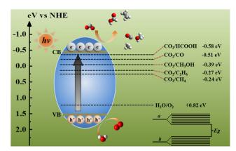
Fig. 1 The fundamentals of photocatalytic CO<sub>2</sub> reduction
