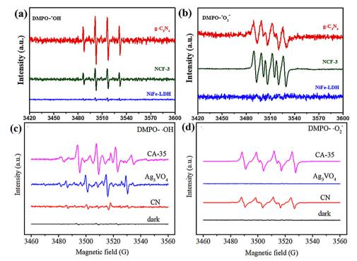
Fig. 21 The ESR spectrum of the type-II g-C<sub>3</sub>N<sub>4</sub> foam/LDH photocatalyst (a and b) and Z-Scheme g-C<sub>3</sub>N<sub>4</sub>/Ag<sub>3</sub>VO<sub>4</sub>/r-GO photocatalyst (c and d) (Figures taken with permission from ref. 182 and 117 copyright 2023, Elsevier).
