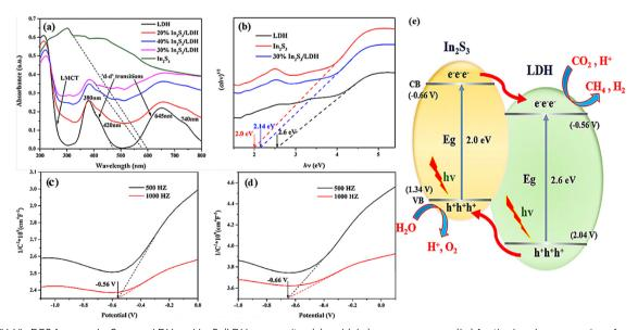
Fig. 16 UV-Vis DRS for pure  $In_2S_3$ , pure LDH and  $In_2S_3/LDH$  composites (a) and  $(\alpha h \nu)_{1/2}$  versus energy  $(h \nu)$  for the band gap energies of pure  $In_2S_3$  and pure LDH (b), Mott-Schottky plots measured for pristine LDH (c) and In<sub>2</sub>S<sub>3</sub> and (d and e) CO<sub>2</sub> photoreduction mechanism on the In<sub>2</sub>S<sub>3</sub>/LDH composites (Figures taken with permission from ref. 74 copyright 2023, ACS).
