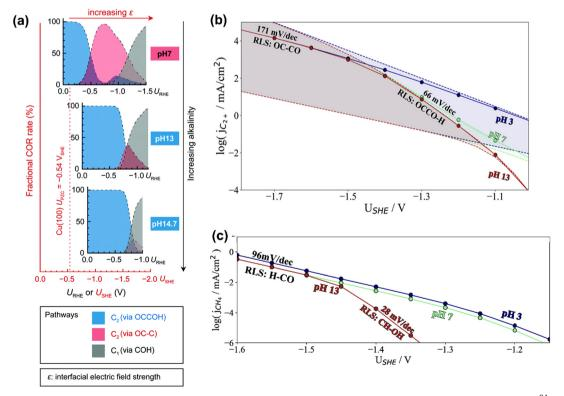
Fig. 3 (a) Product distributions of CO electroreduction on Cu(100) under different bulk pH conditions. Reproduced with permission.<sup>84</sup> Copyright 2021, from RSC Publishing. (b) Simulated current densities using a microkinetic model based on the DFT-calculated energetics on Cu(100). (c) Simulated current densities using a microkinetic model based on the DFT-calculated reaction energetics on Cu(211). Reproduced with permission.<sup>86</sup> Copyright 2022, American Chemical Society.
