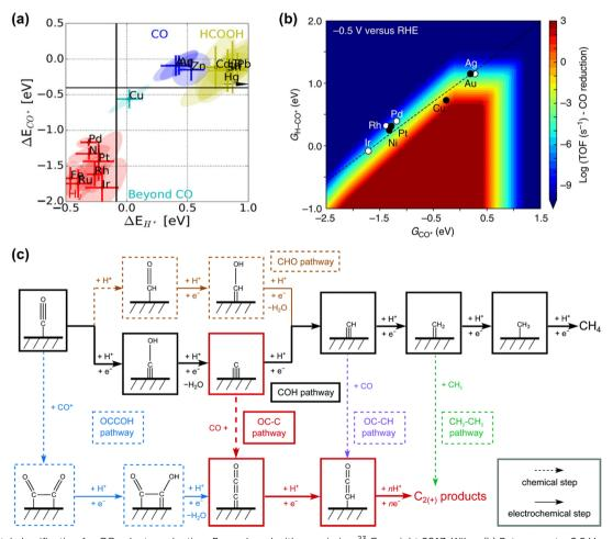
Fig. 2 (a) Metal classification for CO<sub>2</sub> electroreduction. Reproduced with permission.<sup>23</sup> Copyright 2017, Wiley. (b) Rate map at -0.5 V versus reversible hydrogen electrode (RHE) for CH<sub>4</sub> formation over Cu. Reproduced with permission. 82 Copyright 2017, Nature. (c) Schematic diagram of reaction steps for C<sub>2+</sub> over Cu. Reproduced with permission.<sup>84</sup> Copyright 2021, from RSC Publishing
