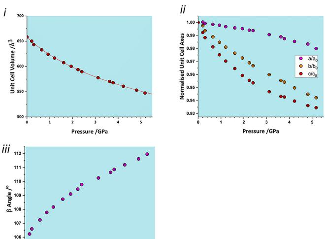
Fig. 3 i) The unit cell volume as a function of pressure. A Birch-Murnaghan 3rd order equation of state has been fitted to yield a bulk modulus of 14.8(4) GPa. ii) Normalised unit cell axes lengths as a function of pressure. iii)  $\beta$  angle as a function of pressure. Error bars are plotted for all parameters but are mostly smaller than the data symbols.
