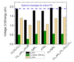
Fig. 2 Optical bandgap, experimentally obtained  $V_{\rm OC}$ , and voltage losses of PIM-based IPVs.
