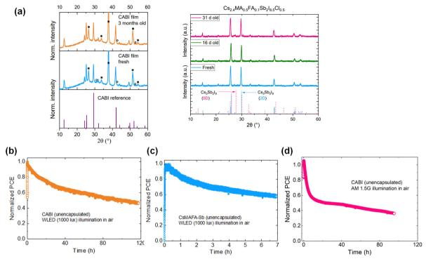
Fig. 4 (a) XRD patterns of fresh and aged CABI films stored in air (reproduced from<sup>24</sup>) and fresh and aged CsMAFA-Sb films stored in dry air (RH of 15%) (reproduced from 31). MPP tracking of unencapsulated devices (in their n-i-p planar device architecture) of (b) CABI and (c) CsMAFA-Sb under WLED (1000 lux) illumination, and (d) CABI under 1-Sun illumination in air (RH  $\sim$ 50%)
