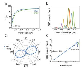
Fig. 2 (a) UV-vis-NIR transmittance spectra of  $\it R-/S-Zn$ . (b) Wavelength-dependent SHG intensities of  $\it R-Zn$  at various excitation wavelengths from 800 to 1040 nm. (c) Polarization dependence of the SHG intensity from the  $\it R-Zn$  crystal under the excitation of 960 nm. (d) Logarithmic plot of SHG intensity as a function of the incident power.
