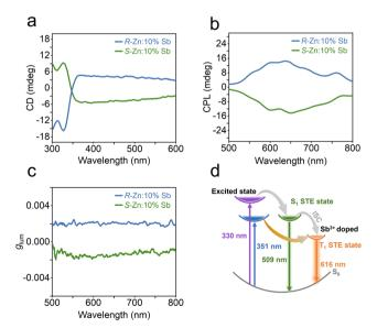
Fig. 4 (a) CD spectra, (b) CPL spectra and (c) corresponding  $g_{lum}$  of R-/S-Zn:10%Sb. (d) Schematic illustration of the proposed PL process in R-Zn:x%Sb
