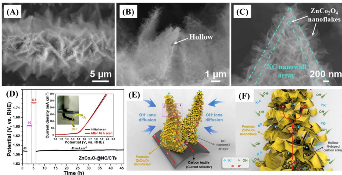
Fig. 22 (A–C) SEM images of  $\text{ZnCo}_2\text{O}_4/\text{NC}/\text{CT}$ . (D) Stability measurements of  $\text{ZnCo}_2\text{O}_4/\text{NC}/\text{CT}$  at different current densities and (E and F) schematic illustration of the  $\text{ZnCo}_2\text{O}_4/\text{NC}/\text{CT}$  electrode. Reproduced with permission.<sup>138</sup> Copyright © 2019 Published by Elsevier B.V.
