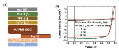
Fig. 4 (a) Device configuration with different thickness of the intrinsic  $C_{60}$  layer and (b) the J-V curve under 100 mW cm<sup>-2</sup> AM1.5 light illumination.
