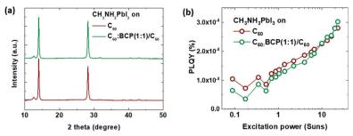
Fig. 5 (a) X-Ray diffraction patterns of  $CH_3NH_3PbI_3$  films grown on  $ITO/C_{60}$  and  $ITO/C_{60}$ :BCP/C<sub>60</sub> and (b) photoluminescence quantum yield (PLQY) under different excitation powers
