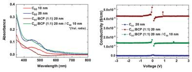
Fig. 2 (a) Absorbance spectra and (b) conductivity vs. applied voltage of mixed C<sub>60</sub>:BCP and pure C<sub>60</sub> films
