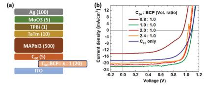
Fig. 3 (a) Device configuration with different composition of the C<sub>60</sub>:BCP mixture (number in parenthesis represent the layer thickness in nm) and (b) the J-V curve under 100 mW cm<sup>-2</sup> AM1.5 light illumination.
