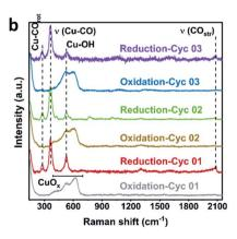
Fig. 4 In situ Raman studies on oxidized Cu species of Cu/PTFE. (a) In situ SERS of Cu/PTFE conducted at different times of reaction in KHCO<sub>3</sub> electrolyte at a current density of 30 mA cm<sup>-2</sup>. (b) The structure and surface adsorbates during reduction and oxidation cycles at 0.6 mA cm<sup>-2</sup> oxidation current density for 20 s.
