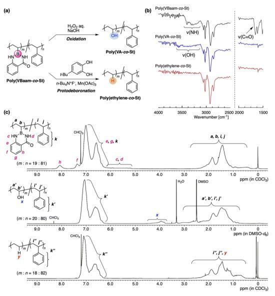
Fig. 4 Transformability of the VBaam unit in the copolymer: (a) C-B bond-cleaving oxidation and protonation. (b) FT-IR and (c) <sup>1</sup>H NMR spectra of poly(VBaam-co-St), poly(vinyl alcohol-co-St), and poly(ethylene-co-St)
