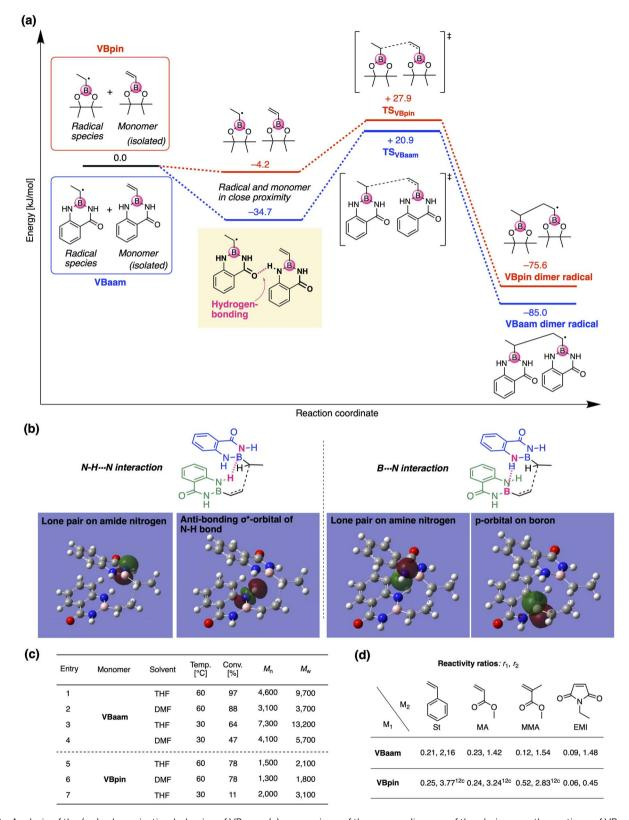
Fig. 3 Analysis of the (co)polymerization behavior of VBaam: (a) comparison of the energy diagram of the chain-growth reactions of VBaam and VBpin, calculated at the (U)CAM-B3LYP/6-31G(d) level. (b) Interactions between two aam groups observed in the NBO calculations. (c) Effect of the conditions on the polymerization of VBaam and VBpin. (d) Monomer reactivity ratios of the boron monomers ( $M_1$ ) in copolymerizations with common vinyl monomers ( $M_2$ ) [ $r_1$  (left),  $r_2$  (right)].
