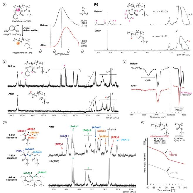
Fig. 5 Synthesis of poly(ethylene-co-TBA) by C-B bond transformation of poly(VBaam-co-TBA); change in the (a) SEC trace and the (b)  $^1$ H NMR and (c)  $^{13}$ C NMR spectra. (d) A comparison of the aliphatic region in the  $^{13}$ C NMR spectra of poly(ethylene-co-TBA) and the TBA homopolymer (the asterisk denotes the peak from the t-butyl group of a very small amount of TBC). (e) Change in the IR spectra due to protodeboronation. (f) DSC curves of poly(ethylene-co-TBA) and TBA homopolymer.
