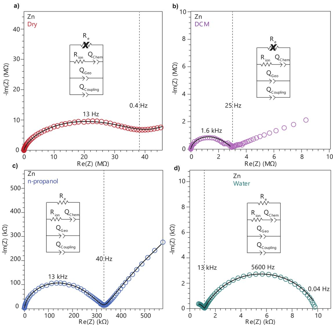
Fig. 4 Nyquist plots of  $\text{TMA}_2\text{ZnGe}_4\text{S}_{10}$  pressed-pellets when dry (a) and after addition of DCM (b), *n*-propanol (c), and deionized water (d). Black traces represent fits to the equivalent circuit diagrams shown in the figure. Crossed-out circuit elements denote elements that are too large to adequately fit to the impedance response.
