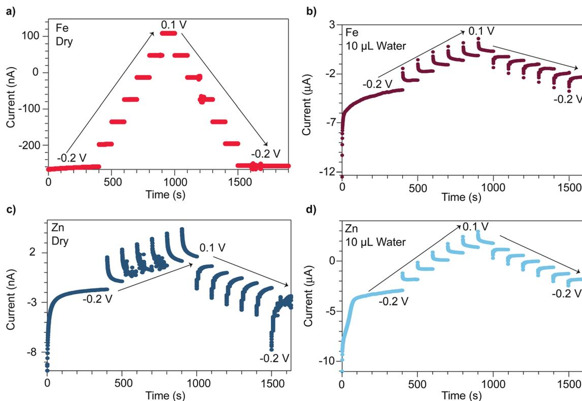
Fig. 1 Chronoamperometry traces of  $\text{TMA}_2\text{FeGe}_4\text{S}_{10}$  and  $\text{TMA}_2\text{ZnGe}_4\text{S}_{10}$  pressed-pellets under applied voltages spanning  $-0.2$  V to  $0.1$  V when dry (a and c), and after treatment with  $10\ \mu\text{L}$  of deionized water (b and d), respectively.
