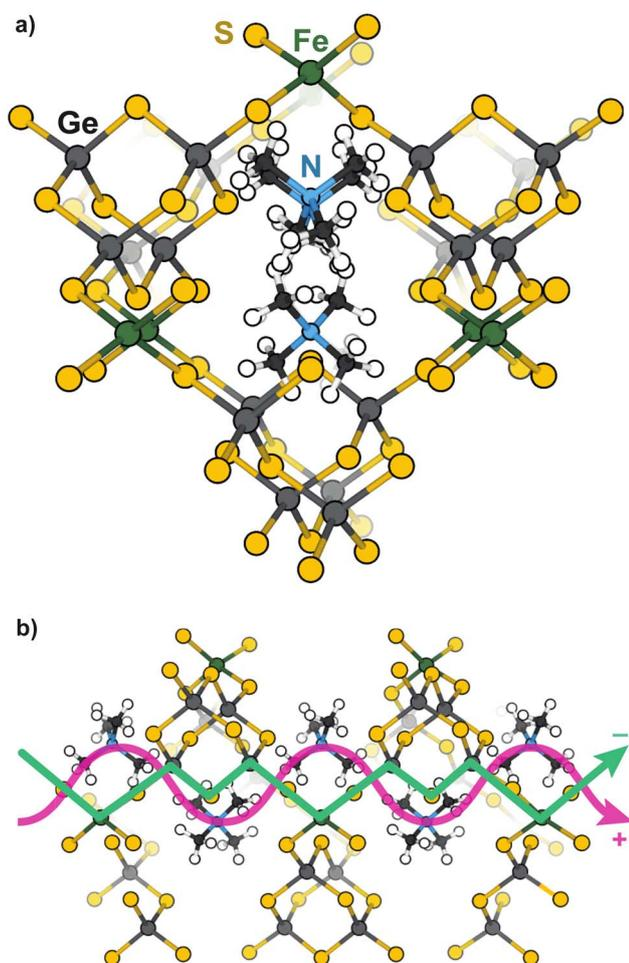
Scheme 1 Representations of  $\text{TMA}_2\text{FeGe}_4\text{S}_{10}$  viewed along the (a) [100] and (b) [101] directions. Proposed conduction pathways of delocalized electrons and extra-framework cations are highlighted in green and pink, respectively.
