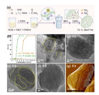
Fig. 1 (a) Schematic diagram of the PAM-assisted synthesis of TS-1 zeolite, (b) relative crystallinity of TS-1 samples crystallized at 80 °C for 3 h and then at 120 °C for different time, TEM images of P-10-80-120 crystallized at 120 °C for (c) 2 h and (d) 3 h, and P-0-80-120 crystallized at 120 °C for (e) 6 h and (f) 8 h, and (g) AFM image of P-0-80-120 crystallized at 120 °C for 8 h.
