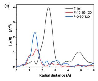
Fig. 4 (a) UV-vis spectra, (b) Ti K-edge XANES spectra, and (c) Fourier transform  $k^2$ -weighted Ti EXAFS spectra in the R spacing of P-0-80-120 and P-10-80-120
