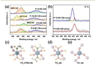
Fig. 5 (a) XPS spectra of Ti 2p in P-10-80-120 and P-0-80-120 before and after calcination, (b) XPS spectra of N 1s of P-10-80-120 and P-0-80-120 before calcination and proposed titanium active sites: (c) TiO $_6$  (PAM) site, (d) TiO $_6$  site and (e) TiO $_4$  site.
