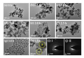
Fig. 2 TEM images of P-10-80-120 samples crystallized at 80  $^{\circ}$ C for 3 h and then at 120  $^{\circ}$ C for (a) 0 h, (b) 0.5 h, (c) 1.0 h, (d) and (h) 1.5 h, (e) 2.0 h, (f) 2.5 h, and (g) 3.0 h (scale bar = 200 nm, especially, 100 nm for (g)), and SAED images of (i) area I and (j) area II.
