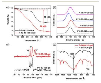
Fig. 3 (a) TG curves of P-10-80-120 and P-0-80-120 before calcination, (b) XPS spectra of Si 2p of P-10-80-120 and P-0-80-120 before and after calcination, (c)  $^{29}$ Si MAS NMR spectra and (d) FT-IR spectra of the P-0-80-120 gel and P-10-80-120 gel.
