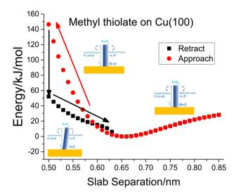
Fig. 1 Plot of the energy *versus* slab separation for the compression of a vertical methyl thiolate species on Cu(100) as a function of the distance from a hydrogen-atom-covered Cu(100) surface for the approach of the two slabs (•) until the initially vertical methyl thiolate species tilts. The structural changes associated with the approach and retraction of the slabs is shown in movie S3.† Shown also are cartoons that illustrate the onset of critical buckling.
