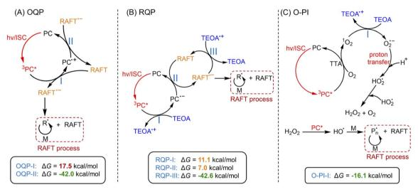
Scheme 2 Proposed mechanism of photo-RAFT polymerization catalyzed by  $ZnPCS_4^-$  via three pathways. A Note: A Note:
