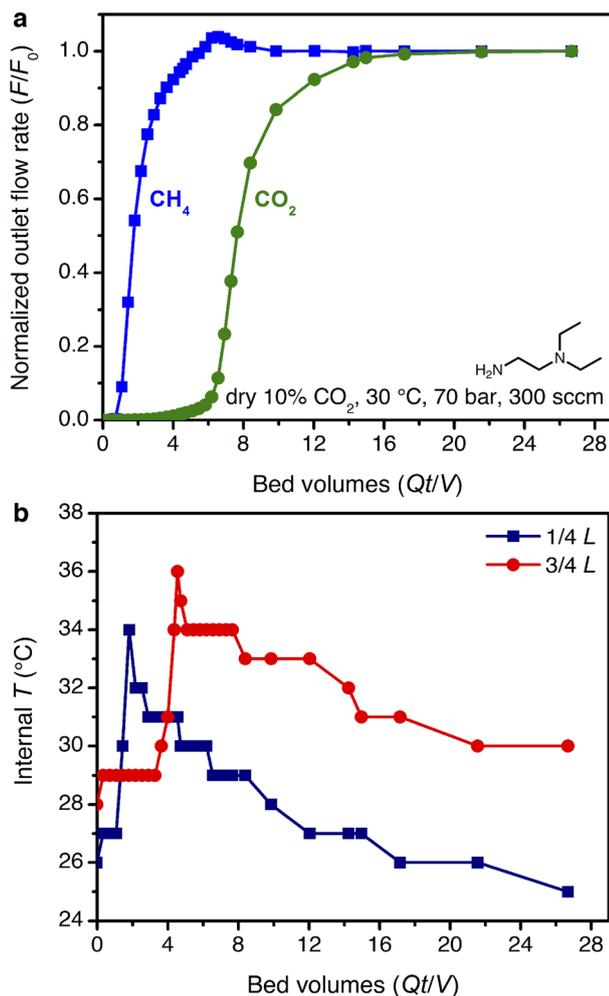
Fig. 6 (a) Breakthrough profile for ee-2-Mg<sub>2</sub>(dobpdc) under 300 sccm of dry 10% CO<sub>2</sub> in CH<sub>4</sub> at 70 bar and 30 °C. (b) Corresponding temperature profile, as measured with two internal thermocouples.
