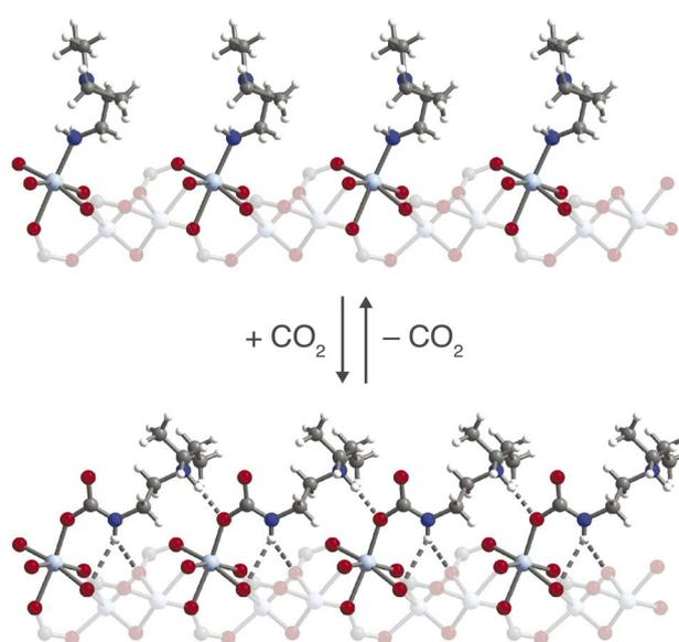
Fig. 8 Structure of ee-2-Zn<sub>2</sub>(dobpdc) before (top) and after (bottom) CO<sub>2</sub> insertion to form ammonium carbamate chains, as observed by single-crystal X-ray diffraction. Light blue, blue, red, gray, and white spheres represent Zn, N, O, C, and H atoms, respectively. The structure of ee-2-Zn<sub>2</sub>(dobpdc) prior to CO<sub>2</sub> adsorption was obtained from ref. 31.
