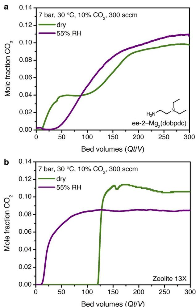
Fig. 7 Dry (green) and humid (purple, 55% RH, second cycle) qualitative breakthrough curves for (a) ee-2-Mg<sub>2</sub>(dobpdc) and (b) zeolite 13X. Humidity eliminates CO<sub>2</sub> slip for ee-2-Mg<sub>2</sub>(dobpdc) and generates a five-fold increase in breakthrough volume, while zeolite 13X shows an eight-fold decrease in breakthrough volume under humid conditions. Materials were evacuated at 30 °C with a vacuum pressure of 0.02 mbar for 12 h between cycles.
