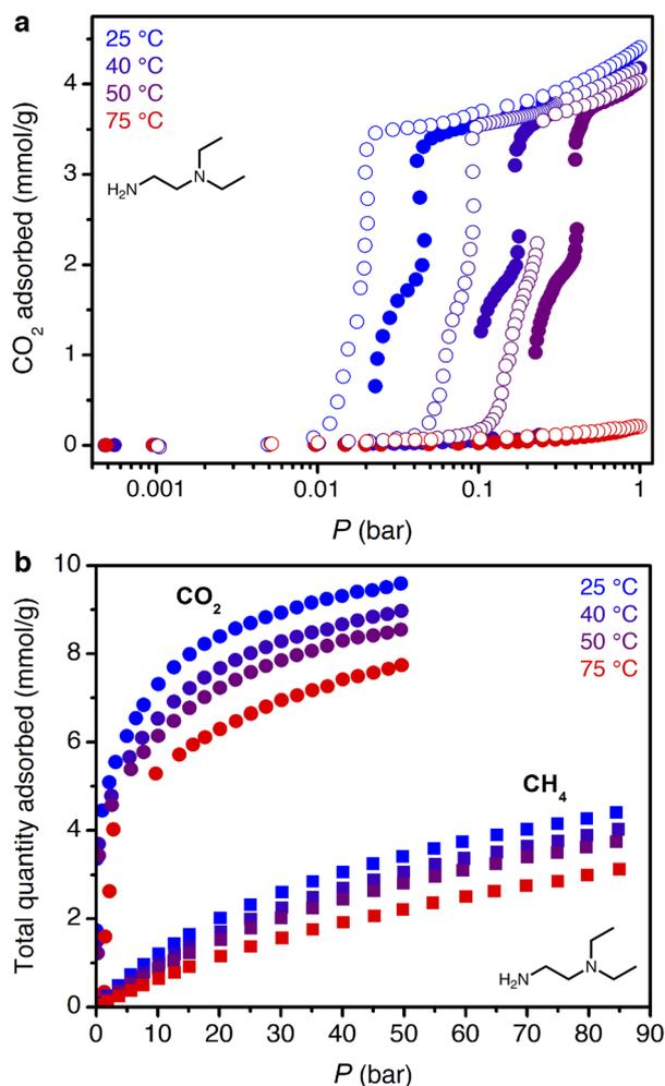
Fig. 5 (a) Low-pressure CO<sub>2</sub> adsorption (filled circles) and desorption (open circles) isotherms for ee-2-Mg<sub>2</sub>(dobpdc). (b) High-pressure CO<sub>2</sub> (circles) and CH<sub>4</sub> (squares) adsorption isotherms for ee-2-Mg<sub>2</sub>(dobpdc).
