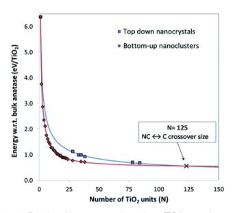
Fig. 3 Energies of bottom-up and top-down ( $TiO_2$ ) $_n$  nanoclusters with the corresponding fitting lines. The NC  $\leftrightarrow$  C crossover size is indicated by the cross at n=125 (i.e., 375 atoms). Reproduced from ref. 20 with permission from the Royal Society of Chemistry.
