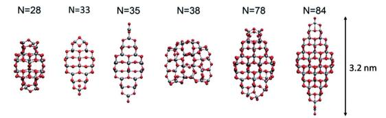
Fig. 2 Atomic structures of the top-down (TiO<sub>2</sub>)<sub>n</sub> nanocrystals investigated in ref. 20. The scale bar on the right strictly refers to the larger model. Titanium, red; oxygen, grey. Reproduced from ref. 20 with permission from the Royal Society of Chemistry.
