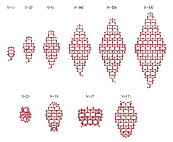
Fig. 4 The octahedral (top) and cuboctahedral (bottom) (TiO<sub>2</sub>)<sub>n</sub> nanoparticles investigated in ref. 21. Reprinted with permission from O. Lamiel-Garcia, K. C. Ko, J. Y. Lee, S. T. Bromley and F. Illas, *J. Chem. Theory Comput.*, 2017, 13, 1785–1793. Copyright 2017 American Chemical Society.
