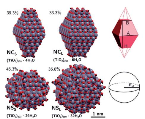
Fig. 9 Top: faceted  $TiO_2$  NPs and a corresponding schematic representation of the Wulff-shape decahedron. Bottom: spherical  $TiO_2$  nanoparticles and a corresponding schematic representation of the sphere. The surface-to-bulk percentage ratio and stoichiometry are also shown. Reprinted with permission from G. Fazio, L. Ferrighi and C. Di Valentin, *J. Phys. Chem. C*, 2015, **119**, 20735–20746. Copyright 2015 American Chemical Society.
