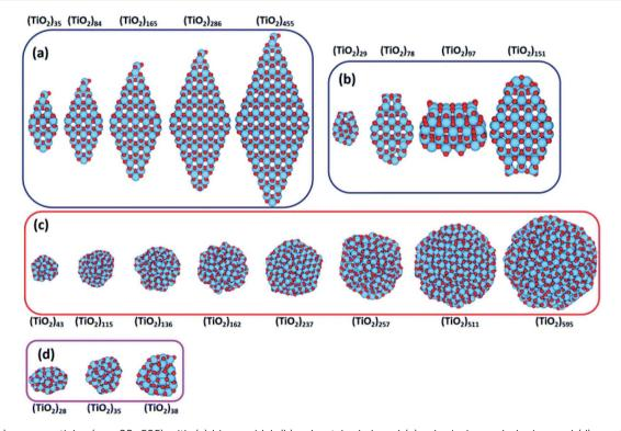
Fig. 6 ( $TiO_2$ )<sub>n</sub> nanoparticles (n = 28-595) with (a) bipyramidal, (b) cuboctahedral, and (c) spherical morphologies, and (d) quasi-spherically globally optimised structures investigated in ref. 42. Red/blue spheres correspond to O/Ti atoms. Reproduced from ref. 42 with permission from the Royal Society of Chemistry.
