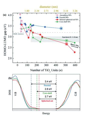
Fig. 8 (a) Optical gap estimated as the HOMO-LUMO difference for faceted (blue), spherical cut (red), annealed core-shell spherical (green), and amorphous (magenta)  $(\text{TiO}_2)_n$  nanoparticles as a function of n. (b) The density of state (DOS) of faceted  $(\text{TiO}_2)_{455}$  and relaxed direct cut and annealed spherical  $(\text{TiO}_2)_{511}$  nanoparticles—corresponding to the circled data points in (a). Reproduced from ref. 42 with permission from the Royal Society of Chemistry.
