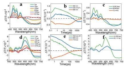
Fig. 3 (a-c) fs-TA spectra at different delay times, the dynamic curve at different wavelengths and the evolution-associated spectra obtained through global fitting of EH-Fla. (d-f) fs-TA spectra at different delay times, the dynamic curve at different wavelengths and the evolution-associated spectra obtained through global fitting of TIPS-Fla.
