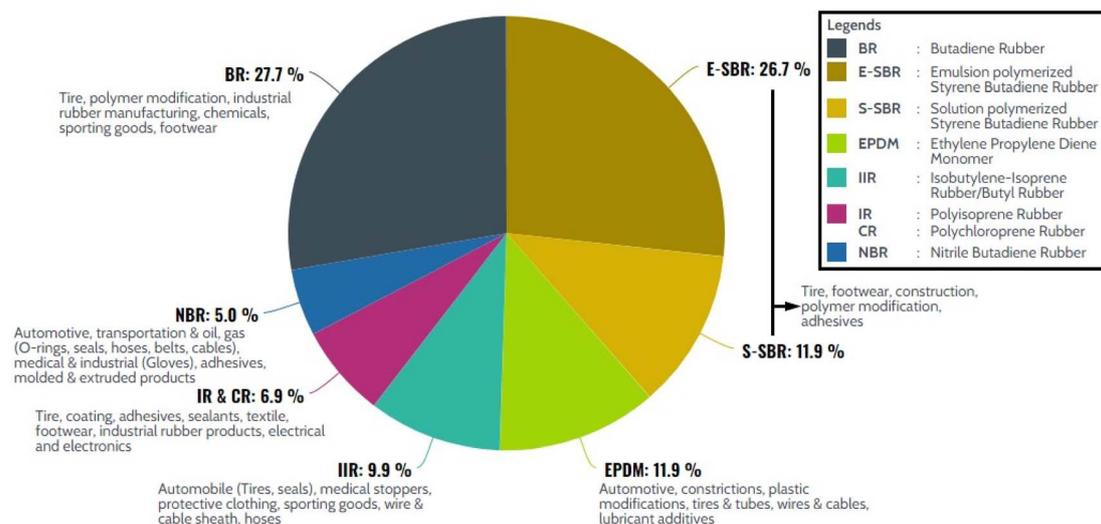
Fig. 4 Demand for synthetic rubber in 2020 according to rubber types, and their respective applications.<sup>49–57</sup>
