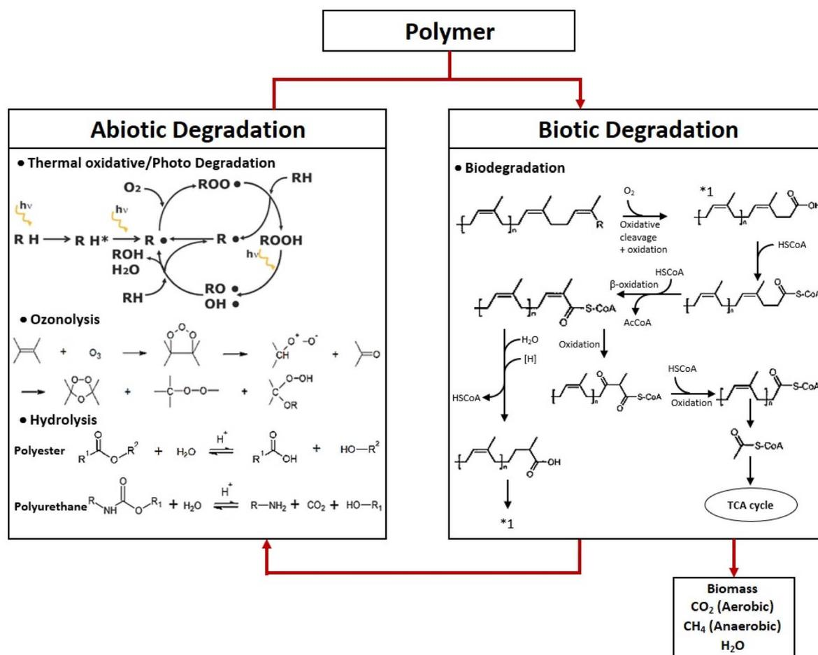
Fig. 6 Mechanisms of various environmental degradation of polymeric materials.<sup>114–116</sup>
