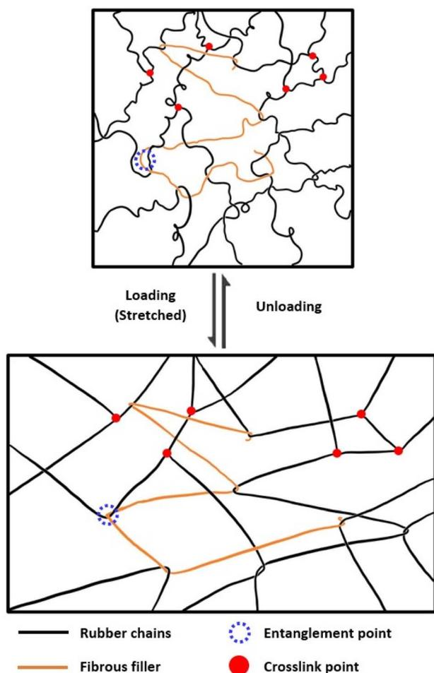
Fig. 7 Mechanical strength reinforcement by fibrous fillers through physical entanglement.<sup>117</sup>
