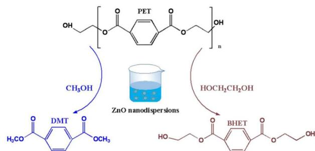
Fig. 11 Nano-ZnO dispersion catalyzed depolymerization of PET.
