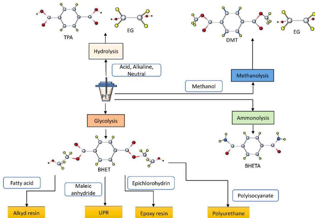
Fig. 3 Chemical recycling process of waste PET.
