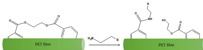
Fig. 8 Decomposition reaction of PET with amine-based molecules.<sup>27</sup>
