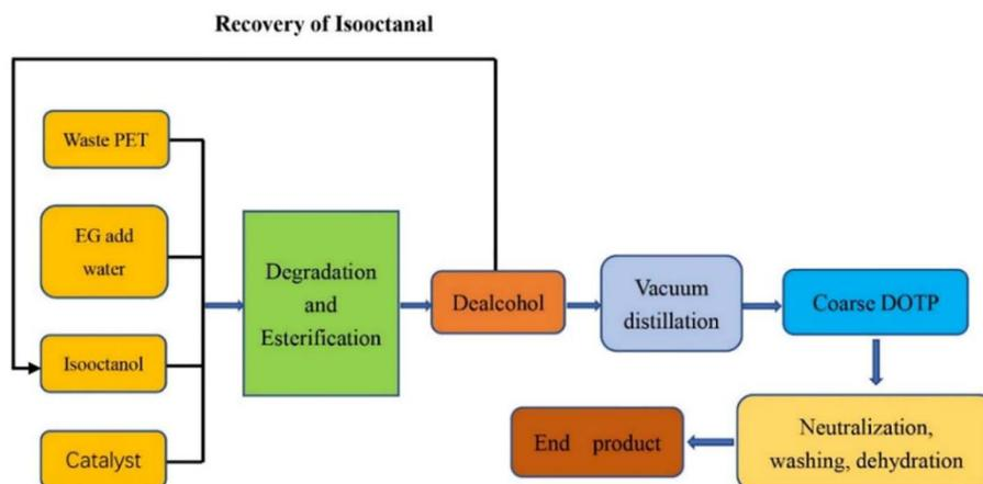
Fig. 13 DOTP made from waste PET.
