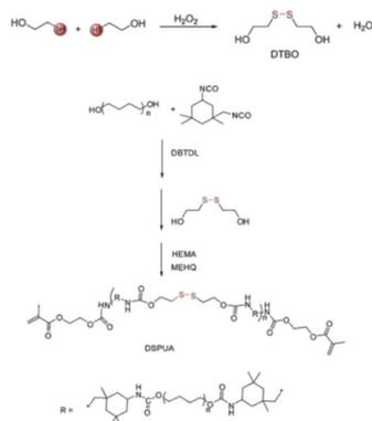
Fig. 1 Synthesis of self-healing UV-curable coating containing disulfide bonds. This figure has been adapted from ref. 24 with permission from Elsevier, copyright 2019.
