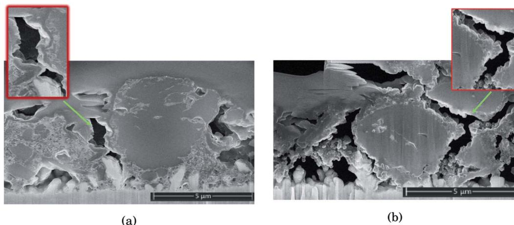
Fig. 2 Comparison of cross sections in Si electrodes after 10 cycles in (a) 1 M LiFSI and (b) 1 M LiPF<sub>6</sub>. A layer of carbon has been coated on the electrode surface to protect the electrode structure beneath from the ion beam during sputtering.
