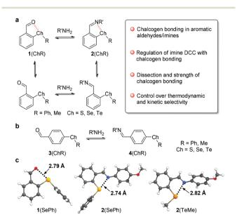
Fig. 1 (a) Illustration of the interplay between the chalcogen bond and dynamic imine chemistry. (b) Structures of control compounds and their imines. (c) Crystal structures of 1(SePh), 2(SePh), and 2(TeMe). The distances of chalcogen bonds are listed.
