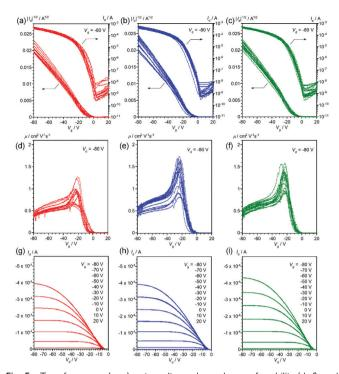
Fig. 5 Transfer curves (a-c), gate-voltage-dependence of mobility (d-f), and output curves (q-i) of OFET devices based on spin-coated R- (red), S- (blue), and rac- (green) EH-DNTT thin films, respectively. Transfer and gate-voltagedependent mobility curves are overlaid for more than twelve devices.
