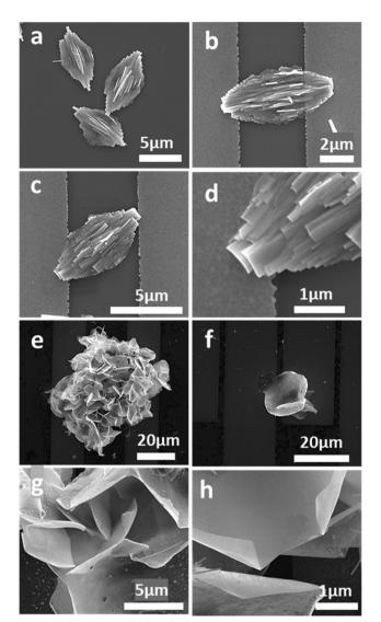
Fig. 3 SEM image of (a) several ZNLs, (b and c) a single ZNL connecting two gold electrodes, (d) at high magnification of a single ZNL, (e-h) SEM images at different magnifications of ZNLs.
