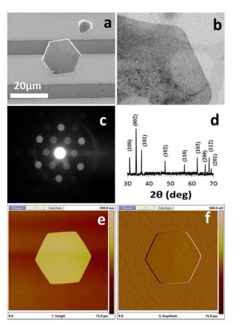
Fig. 2 (a) SEM image, (b) the corresponding SAED pattern, (c) STEM image, (d) the XRD pattern, (e), and (f) AFM images of the ZNDs.
