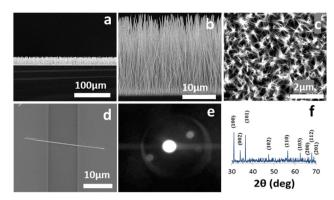
Fig. 1 (a) Low magnification side view SEM image, (b) high magnification side view SEM image, (c) top view SEM image of an array of ZNWs; (d) SEM image of a single ZNW, (e) the corresponding SAED pattern of the ZNWs, and (f) the XRD pattern of the ZNWs.
