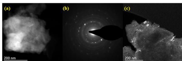
Fig. 3 (a) HADF-STEM image of C50 carbon. (b) SAED pattern acquired over an area of 200 nm. (c) HADF-STEM image of the C-50 sample selecting the reflection at  $d = 0.31 \text{ nm}$  in the SAED pattern.
