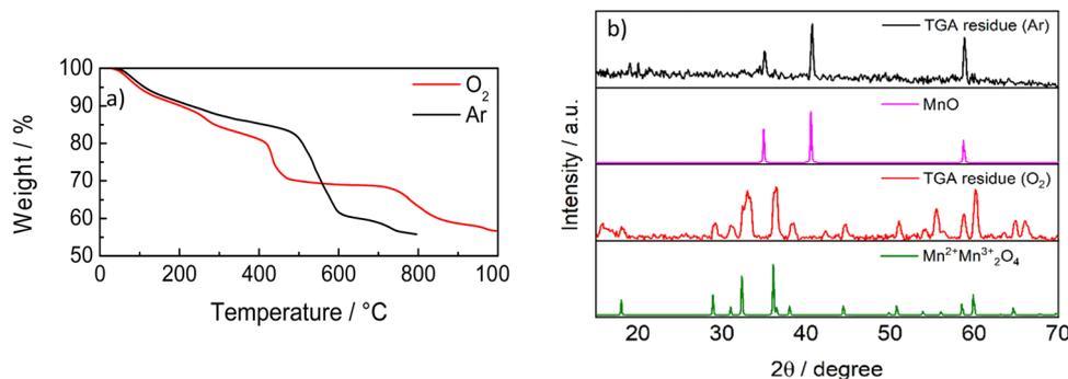
Fig. 6 (a) TGA curves of C-50 in Ar and O<sub>2</sub> at 10 °C min<sup>-1</sup>. (b) XRD patterns of the residues from the TGA of Fig. 6a, MnO (reference code 01-075-0626) and Mn<sub>3</sub>O<sub>4</sub> (reference code 01-089-4837).
