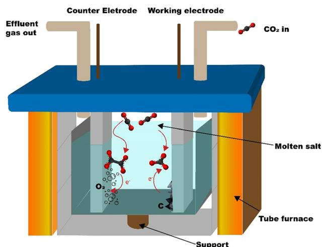
Fig. 1 Schematic of the MSCC-ET reactor.
