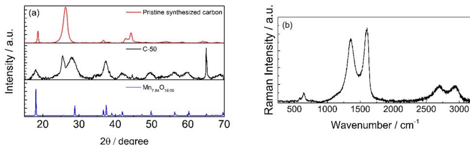
Fig. 4 (a) X-ray diffraction patterns of pristine synthesized carbon (red), C-50 (black) and diffractogram of  $\text{Mn}_{7.84}\text{O}_{16}$  (reference code 96-151-4117). (b) Raman spectrum of the carbon ground in an agate mortar.
