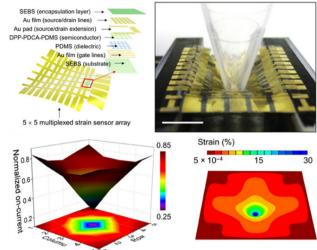
Fig. 13 Architecture, photograph, normalized on-current, and simulation results of strain applied by poking with a plastic bar to the fully stretchable active-matrix TFT array containing self-healable semiconducting polymer.31 Copyright: 2019, Science Advances.
