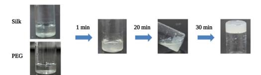
Fig. 7 Gelation process after mixing equal volume of SF and PEG400 solutions at room temperature. Reproduced with permission from Elsevier.<sup>101</sup>
