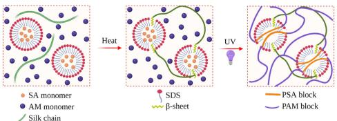
Fig. 14 Preparation of IPN hydrogels composed of SF and poly(acrylamide-co-stearyl acrylate). Reproduced with permission from Wiley-VCH, copyright 2019.163
