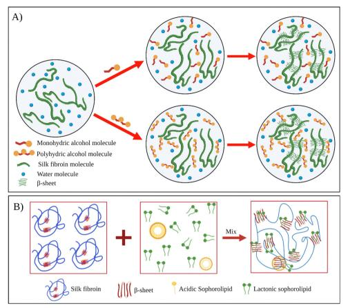
Fig. 5 (A) Schematic illustration of silk fibroin gelation *via* monohydric and polyhydric alcohols. Reproduced with permission from Elsevier,<sup>84</sup> (B) the proposed mechanism of SF gelation induced by sophorolipid molecules. Reproduced with permission from Wiley-VCH, copyright 2015.<sup>91</sup>
