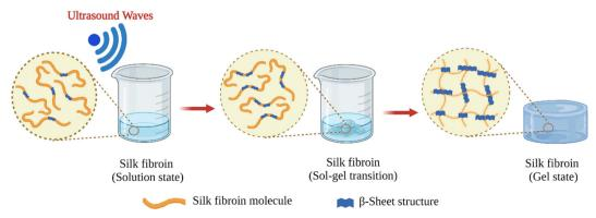
Fig. 8 Schematic illustration of sonication-induced SF gelation
