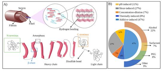
Fig. 4 (A) The structure of SF at different scales. (B) Chart representing the usage of methods to prepare self-assembled SF hydrogels
