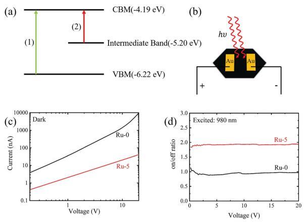
Fig. 5 (a) Schematic illustration of the transition process of the Ru-doping samples. (b) Schematic diagram of the devices. (c) The Volt-Ampere characteristic curves of the devices under dark conditions. (d) On/off ratios of the devices under 980 nm
