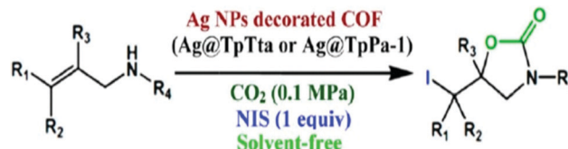
Scheme 31 The synthesis of carbamate using Ag@TpTta/Ag@TpPa-1 COFs. Reproduced with permission from ref. 56; copyright: 2020, ACS Sustainable Chemistry & Engineering.
