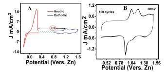
Fig. 3 (A) Voltammogram of zinc and pheno@cnt showing the cell voltage of 1.19 V. (B) Voltammogram showing the excellent stability of the electrode in 100 multiple sweep cycles at a 50 mV s $^{-1}$  scan rate.
