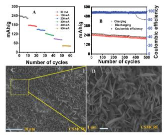
Fig. 7 (A) Rate stability test of the intercalated material at different currents (mA  $g^{-1}$ ). (B) Cycling stability test at 50 mA  $g^{-1}$ . (C) FESEM images of the cathode. (D) The anode after the cycling experiment.
