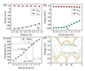
Fig. 4 (a and b) valley-splitting changes versus interlayer distance and biaxial strain, respectively. (c) Curie temperatures changes versus biaxial strain of monolayer MnSe<sub>2</sub>. (d) Band structure of MoTe<sub>2</sub>/MnSe<sub>2</sub> under 5% tensile strain
