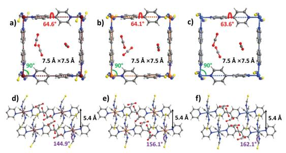
Fig. 5 Comparison of the crystal structures of  $sql-1-M-NCS·3CO_2$ . (a and d) M = Fe; (b and e) M = Co; (c and f) M = Ni
