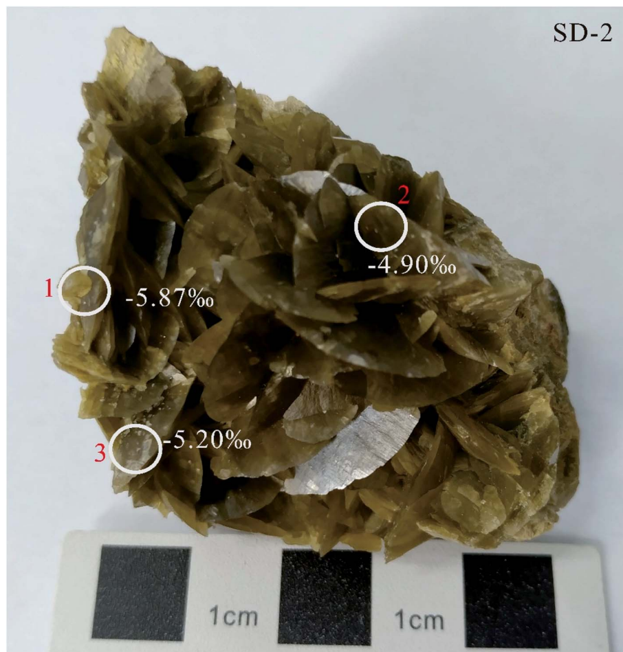
Fig. 2 Photograph of the hand specimen of SD-2 siderite with marked sampling positions of chips 1, 2, and 3 and associated IRMS determined C isotope compositions.
