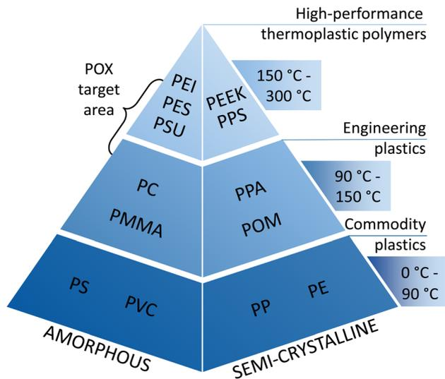
**Fig. 1** Polymer pyramid adapted from de Leon *et al.*, 2021.<sup>9</sup> Temperature ranges given correspond to typical values of heat distortion temperatures and continuous use temperatures of the polymers.<sup>10</sup> For simplicity, only a few polymers are shown by their common abbreviation.
