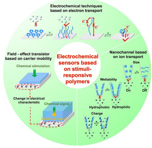
Fig. 7 The sensing principles of stimuli-responsive polymer modified electrochemical sensors.
