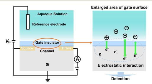
Fig. 10 Structure and principles of Bio-FETs.
