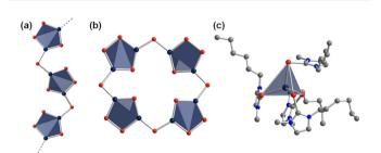
Fig. 3 Infinite zig-zag-strand structure of the anion  $1D-\{[Hg_2Te_4]^2-\}$ (a), molecular structure of the heavy metal porphyranoid anion [Hg<sub>8</sub>Te<sub>16</sub>]<sup>8</sup> (b), molecular structure of the cationic complex [(C<sub>6</sub>C<sub>1</sub>ImTe)<sub>4</sub>Hg]<sup>2+</sup> (c). Hydrogen atoms are omitted for clarity. Color code: Hg-dark blue, Te-red, C-grey, N-blue.
