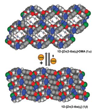
Fig. 2 Space-filing diagrams of the reversible structural transformation between  $1\alpha$  and  $1\beta$  (viewed along the a-axis, for more details see Fig. S5, ESI†).
