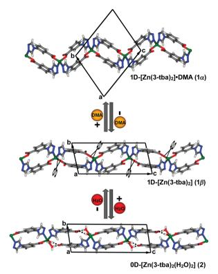
Fig. 1 Structural transformations in  $[Zn(3-tba)_2]$  involving  $1\alpha$ ,  $1\beta$  and 2(unit cells are illustrated). Charge-assisted H-bonding (black broken lines) occurs between agua ligands and free carboxylate moieties in 2.
