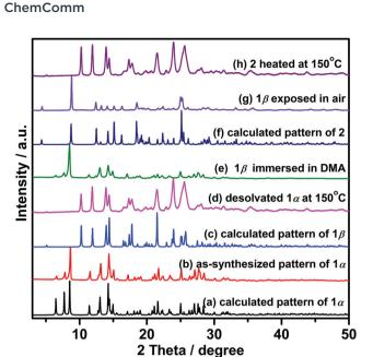
Fig. 3 PXRD patterns of (a)  $1\alpha$  calculated from SCXRD data, (b) assynthesized  $1\alpha$  at room temperature, (c)  $1\beta$  calculated from SCXRD data, (d) desolvated  $1\alpha$  at 150 °C, (e)  $1\beta$  immersed in DMA for 1 day, (f) calculated 2 from SCXRD data, (g)  $1\beta$  exposed to humid air (*ca.* 45% RH), and (h) dehydrated 2 at 150 °C.
