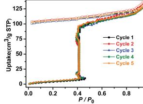
Fig. 5 Five consecutive activation-uptake cycles of water sorption isotherms of  $1\beta$  at 298 K (closed and open symbols denote adsorption and desorption, respectively).
