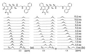
Fig. 2 Aliphatic signals of the  $^{1}$ H NMR spectra of **L1** (a) and **L2** (b) at pH 7 in the presence of increasing amounts of KP. The signal of  $1_{AL}$  is superimposed to the HOD resonance and cannot be confidently monitored ( $D_{2}O/CD_{3}OD$  30:70) (Vol; Vol, [**L1**] =  $1 \times 10^{-2}$  M, 298 K, for **L1**,  $J_{2AL\cdot3AL}$  = 6 Hz; for **L2**,  $J_{2AL\cdot3AL}$  6 Hz;  $J_{3AL\cdot4AL}$  = 7 Hz;  $J_{2AL\cdot4AL}$  cannot be confidently estimated).
