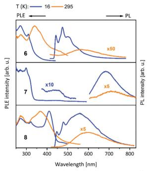
Fig. 6 Solid state excitation and emission spectra of bis-NHCbipy (L2) metal complexes 6-8. PL was excited at  $\lambda_{exc}$  = 300 nm for 6, 8 and  $\lambda_{\rm exc}$  = 320 nm for **7**. PLE spectra were recorded at  $\lambda_{\rm em}$  = 500/560 nm (**6**),  $\lambda_{em}$  = 700/750 nm (7) and  $\lambda_{em}$  = 550/600 nm (8) at low/elevated temperatures respectively.<sup>42</sup>
