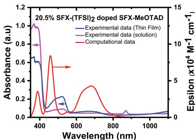
Fig. 8 Comparison of experimental [thin film (blue) and solution (magenta)] and computational absorption spectra (red) for 20.5% SFX-(TFSI)<sub>2</sub> doped SFX-MeOTAD.
