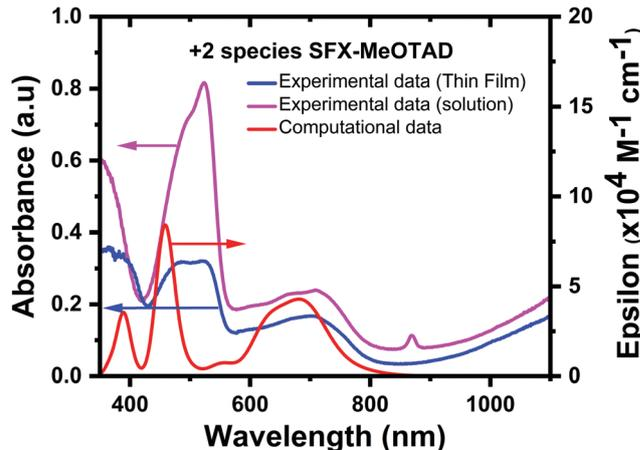
Fig. 6 Comparison of experimental [thin film (blue) and solution (magenta)] and computational absorption spectra (red) for SFX-MeOTAD<sup>2+</sup>.
