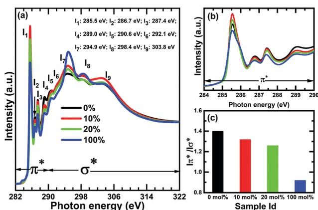
Fig. 10 Comparison of  $C$   $K$ -edge NEXAFS spectra corresponding to SFX-MeOTAD [0%], SFX-MeOTAD doped with 10 mol% SFX(TFSI)<sub>2</sub> [10%], SFX-MeOTAD doped with 20 mol% SFX(TFSI)<sub>2</sub> [20%] and SFX(TFSI)<sub>2</sub> dopant [100%]; (b)  $\pi^*$  resonances at the absorption edge and (c) variation in the  $I_{\pi^*}/I_{\sigma^*}$  ratio for all the samples.
