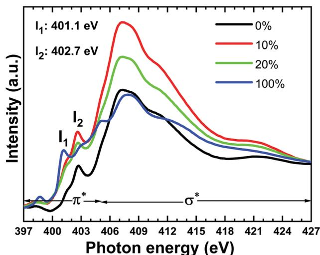
Fig. 11 Comparison of N K-edge NEXAFS spectra corresponding to SFX-MeOTAD [0%], SFX-MeOTAD doped with 10% SFX(TFSI)<sub>2</sub> [10%], SFX-MeOTAD doped with 20% SFX-(TFSI)<sub>2</sub> [20%] and SFX(TFSI)<sub>2</sub> dopant [100%].
