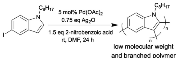
Scheme 10 Room-temperature DARP of 5-iodo-1-octylindole monomer.
