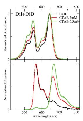
Fig. 4 Absorption and emission spectra (excitation wavelength: 495 nm) of solutions/suspensions of 1:1 Dil/DiD in different environments.
