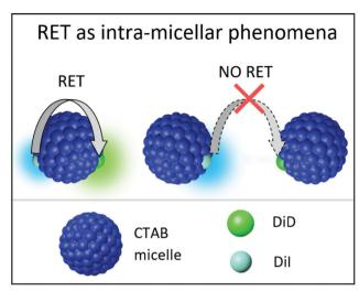
Fig. 5 Schematic representation of RET as intramicellar phenomena when micelles are loaded with Dil and DiD at equimolar ratios
