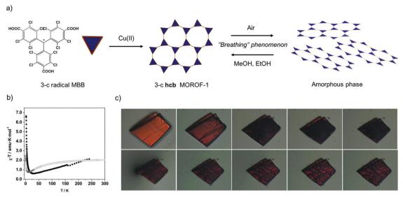
Fig. 4 (a) Schematic representation of the formation of hcb MOROF-1 using the 3-c PTMTC and Cu(ιι), and its breathing behaviour. (b) Value of γT as a function of the temperature for MOROF-1 (filled circle, MOROF-1; open circle, evacuated and amorphous MOROF-1 phase), (c) Breathing phenomenon of a single crystal of MOROF-1 when exposed to the air (top) and re-exposed to ethanol liquid (bottom). (b and c) Adapted from ref. 69. Copyright 2003 Nature Group
